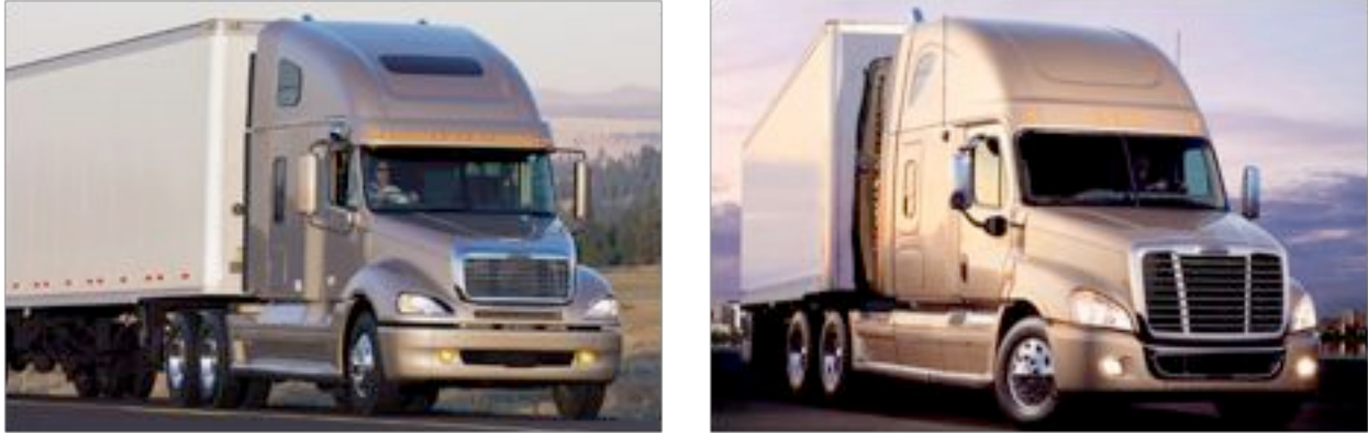
Figure 8: Freightliner Cascadia (right) delivers a 3 percent fuel economy gain over its predecessor, Freightliner Columbia (left).
