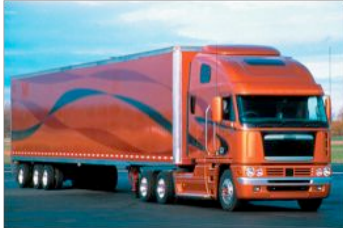
Figure 6: Freightliner Argosy demonstrates a lowered trailer floor & low profile tires
