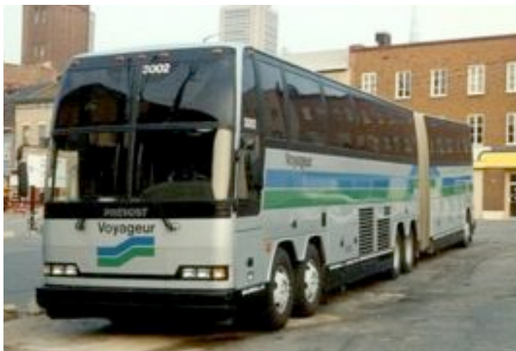
Figure 14: Prevost H5-60 Bus with C_d of 0.384, later reduced to 0.311
